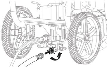
Completely uncoil garden hose or remove completely from reel to prevent kinks.
