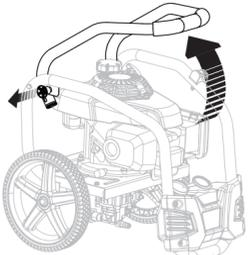
2 Install the trigger handle holder, spray wand holder, and hose storage (see page 7).
