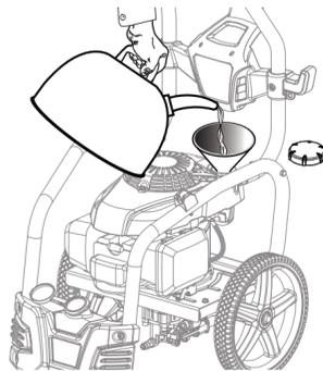
This is a 4-cycle engine. Do not mix fuel and lubricant together.
