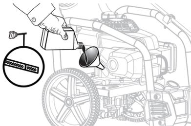
Turn the fuel valve to OFF before adding lubricant.
